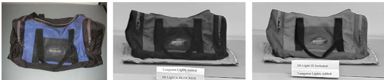
Figure 1. This figure demonstrates differences in the appearance of an object when the camera has a different spectral response. (Left) Color photograph. (Center) Video still from black and white camera with IR blocked out. (Right) Video still from black and white camera with IR allowed to pass.
